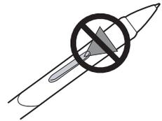
**Important:** Do not remove the switch by prying it from either end as this may damage your Pen. NEVER adjust the trimmer capacitor that will be visible when the switch is removed. When using the pen without the DuoSwitch, always replace the original rubberized grip with the optional grip in order to protect the trimmer capacitor.
