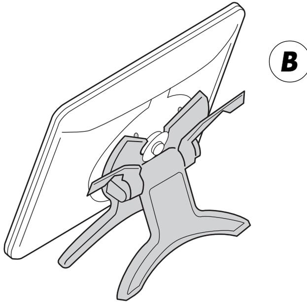
**WARNING** ⚠ When operating the incline adjustment levers, Cintiq must be mounted on the stand with the stand feet resting on a stable, flat surface. The stand is spring-loaded and can snap back quickly, causing injury or damage if not operated properly.
