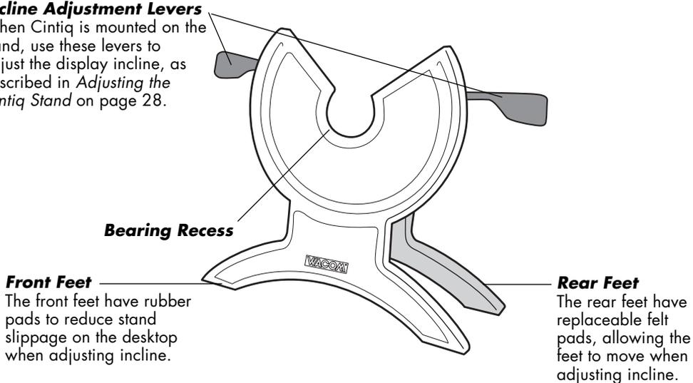
The Cintiq stand supports the Interactive Pen Display unit. The stand can be used to adjust the incline angle of the display unit from a low position (13 degrees from horizontal) to a high position (70 degrees from horizontal). And, you can rotate Cintiq from landscape to portrait orientation, or to any angle between +180 and -180 degrees. The stand also allows easy removal of Cintiq for use in a semi-supported lap position.
