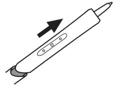
3. Install the optional grip by aligning the pen case rails with the grooves inside the grip and pushing the grip over the pen tip. Then replace the pen tip cone by turning it clockwise onto the pen.
