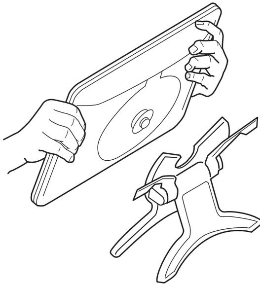
**Note:** When packing Cintiq for transport, always pack the Interactive Pen Display and Cintiq stand in their original containers and protective cushions. Never pack the two items with the display unit mounted on the stand; this may damage the display unit or stand during transportation.
