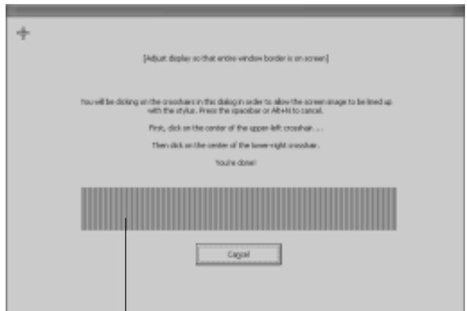
Adjustment pattern for phase and pitch (VGA only).
